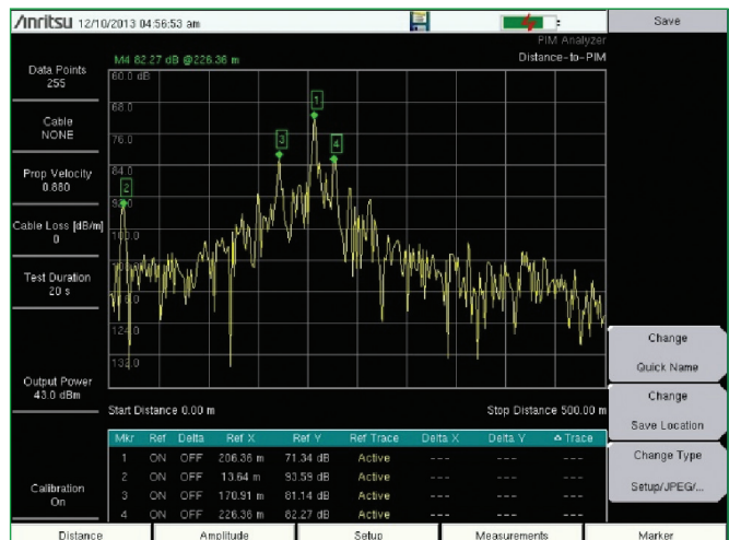
Distance-to-PIM (DTP) measurements from a DAS installation
